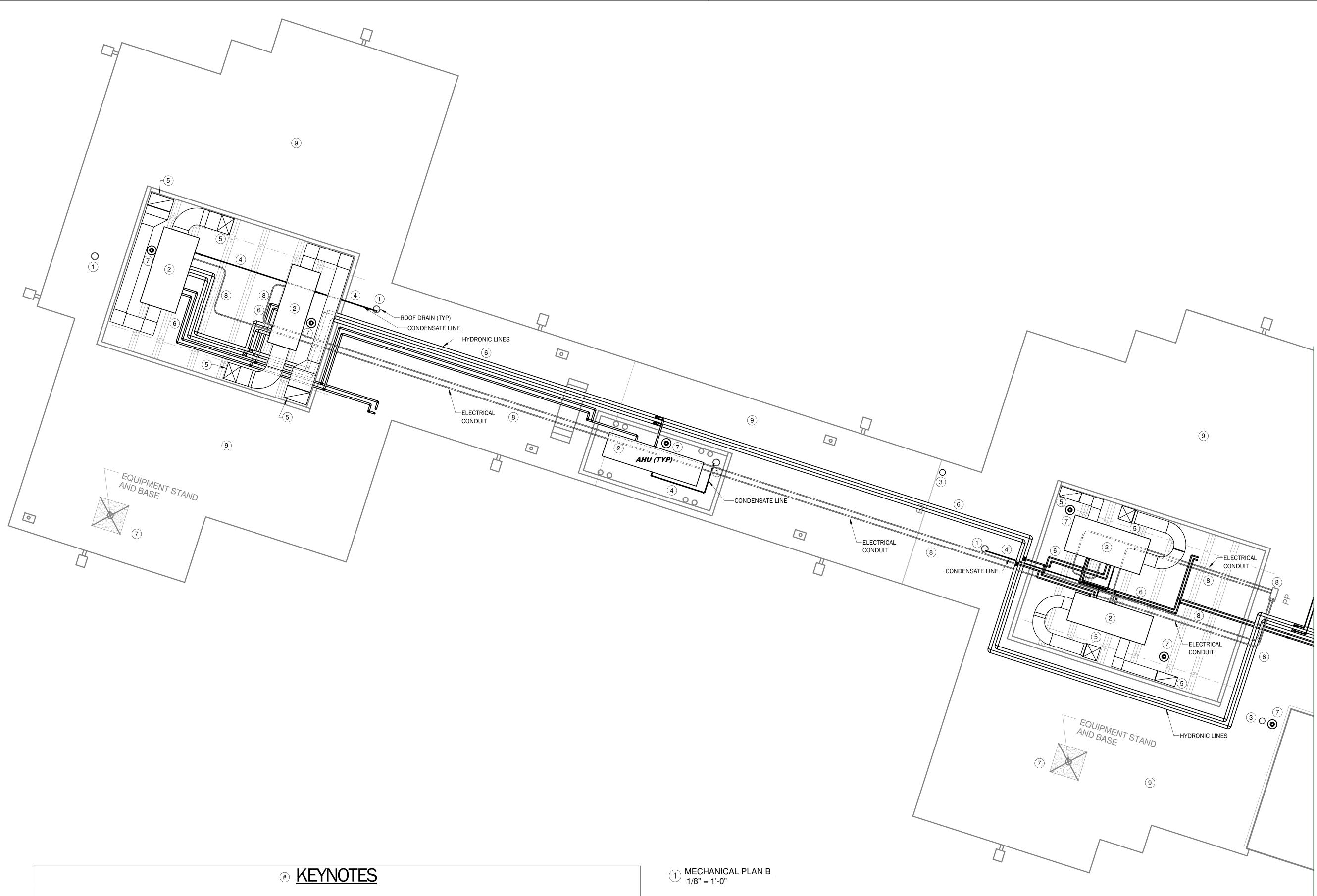
1 EXTEND ROOF DRAIN LEADER THRU NEW ROOF AND CONNECT TO NEW ROOF DRAIN ZURN MODEL Z100 OR APPROVED EQUAL.
